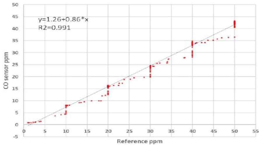
**Figure 3: Correlations between Measurements from CO Reference and Sensor.**
